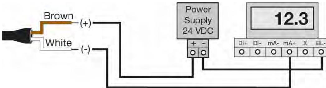
*(Note: the LI23 Series with backlight will have an added 4.5 VDC voltage drop)*
