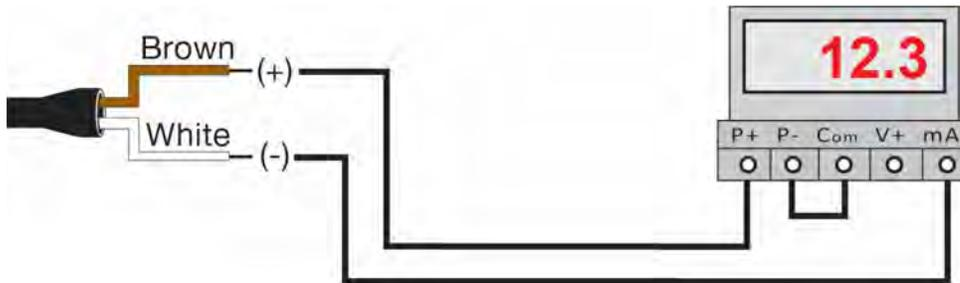
**COMMON WIRING TO DISPLAY, CONTROLLERS AND PLCS:**
