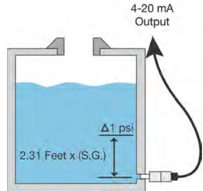
With the above ratio, you can always find the Liquid Height or water column (WC) of any pressure transmitter.
