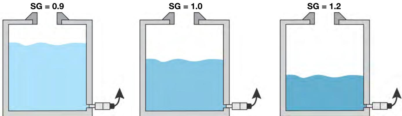
Example: Compare the **Maximum Liquid Height** of a liquid with SG = 0.9, 1.0 and 1.2 using a transmitter with 15 psi pressure range (PR).
