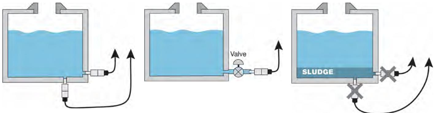
The LD30 series is designed to operate with only the installation thread being exposed to the fluid. Avoid installing the level transmitter along the bottom of the tank as materials such as sludge will build up and coat/cover the port.
