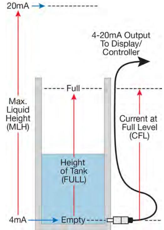
To calculate the **Maximum Liquid Height (MLH)** of a sensor, use the following formulas:
