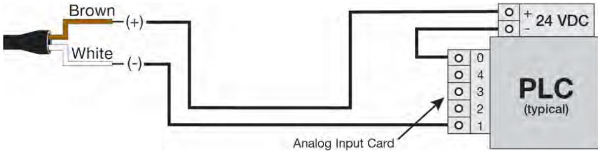
Wiring to the DataView™ LI55 Series Level Controller:
