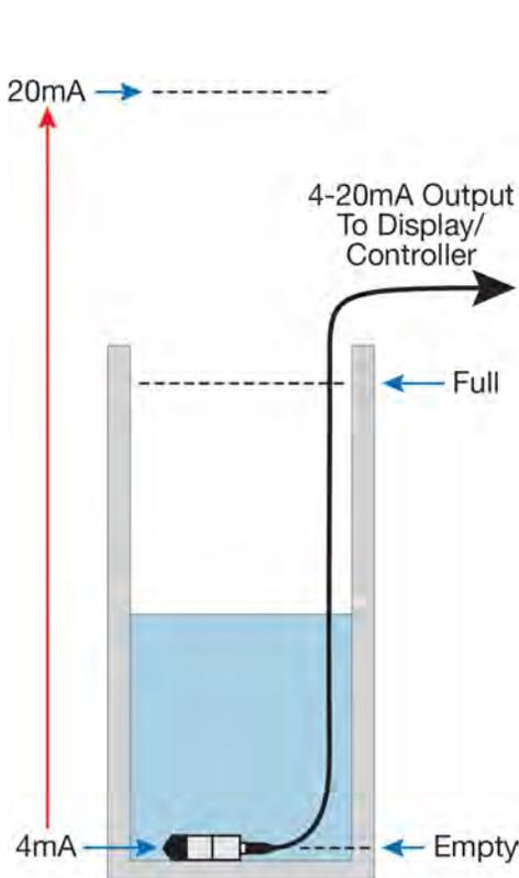
**Sensor offset from Bottom of Tank**
